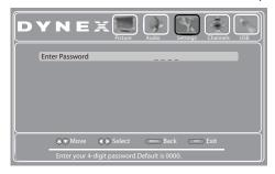
**4** Press the number buttons to enter the four-digit password. The *Parental Controls* menu opens with **Button Lock** highlighted.
